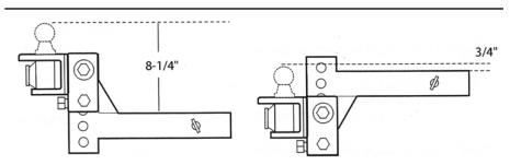
BOLT-TOGETHER BALLMOUNT HAS 7-1/2" ADJUSTMENT, EACH ADJUSTMENT 1-1/4" EXTRA HI-LOW SHANKS AVAILABLE IF NEEDED
