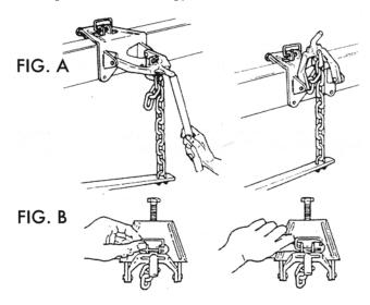
CAUTION: MAKE SURE THAT HOOK-UP ARM IS COMPLETELY SEATED AND SPRING BAR IS PUSHED DIRECTLY UNDER HOOK-UP CHAIN HOOK. Now install Hook-Up locking clip through locking ears and over hook on Hook-Up arm. (See figure B.)
