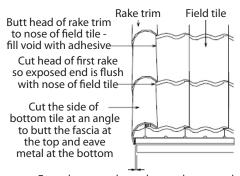
Eave closure and metal extends past end of fascia board and is cut at an angle to support bottom rake at same angle as the rest VariaBlock or Sealant is used to fill any openings
