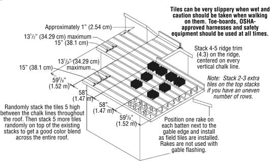
row to be cut on each side. Adjust the starting line to allow for proper rake fit at the gable. Randomly stack Distinction Tile five (5) high between the chalk lines throughout the roof. Then stack five (5) more Distinction Tiles randomly
