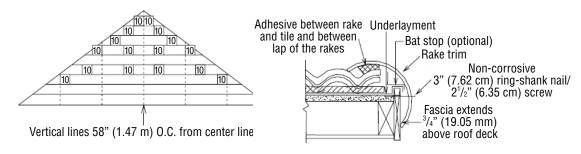
on top of the existing stacks to get a good color blend across the entire roof. Stack four to five (4-5) ridge trim on the ridge, centered on every vertical chalk line. Stack two to three (2-3) extra Distinction Tiles on the top stacks if you have an uneven number of rows. The bottom two battens should be kept free of Distinction Tile stacks. If blending multiple Distinction colors, order an equal amount of each color and blend the colors randomly on the job site for a blended final appearance.
