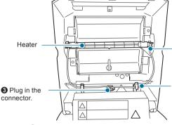
1 Install the heater using the clips.
