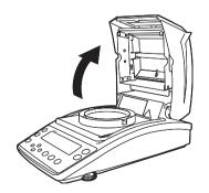
Place a 50-gram calibration weight on the sample pan.
