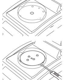
Close the heater cover, and check that the sensor probe fits the indentation in the heater cover.
