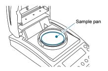
Be sure that (the stability mark) is displayed, and adjust the zero point.
