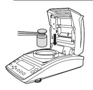
Lower the calibration weight when [0.000] starts to flash.
