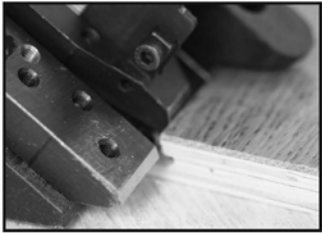
Fig. 18 Pushed in to the groove - correct position
