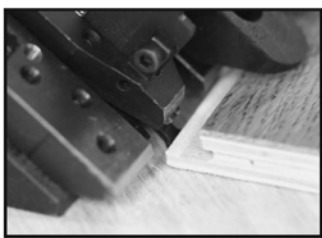
Fig. 15 Pin placed outside locking element - incorrect
