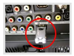
Turn on the TV and insert USB memory drive into "SERVICE" or "WISE-LINK" port on the side or the back of the TV.
