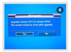
Upgrade will not be performed if new firmware is the same or lower than current version.
