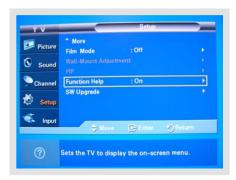
Press "Menu" button and select "Setup" scroll down to select "Function Help" and press "Enter"
