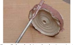
Finally, roll the wheel into the abrasive using light pressure, ensuring a heavy pickup of the abrasive.
